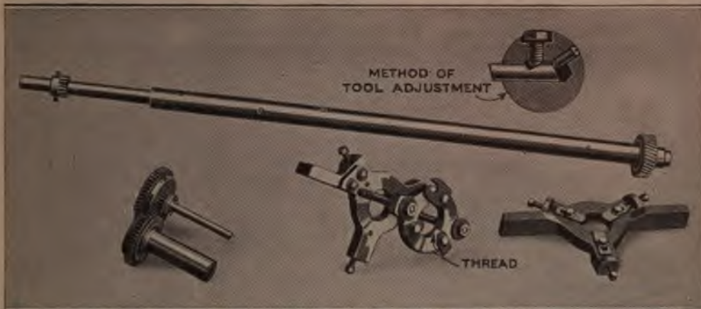
Exploded View of the Apparatus; Above Is the Boring Bar Itself, and in the Insert a View of the Tool Adjustment. To the Left, Below, Is the Train of "Back Gears" through Which the Lead Screw is Driven. In the Center is Seen the Built-Up Nut in Which the Lead Screw Works. To the Right Is One of the Steady Rests
